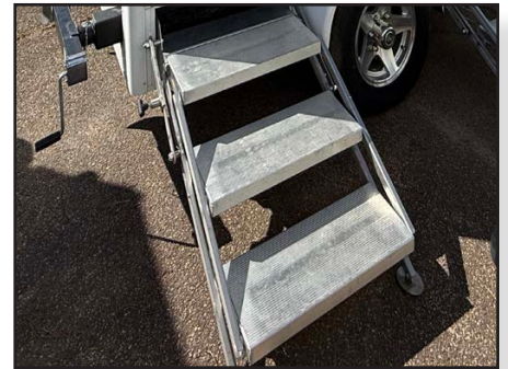
Flip-down steel step assemblies with lighting.
